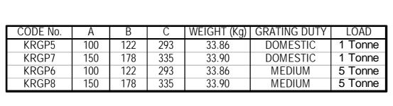
SUPPLIED COMPLETE WITH DOMESTIC OR MEDIUM DUTY GRATE AND GULLY PLUG
