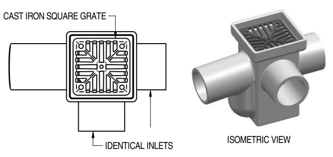
COMPLETE WITH CAST IRON SQUARE GRATE 150 x 150 (6" x 6") CODE KIG2C ALL DIMENSIONS IN mm
