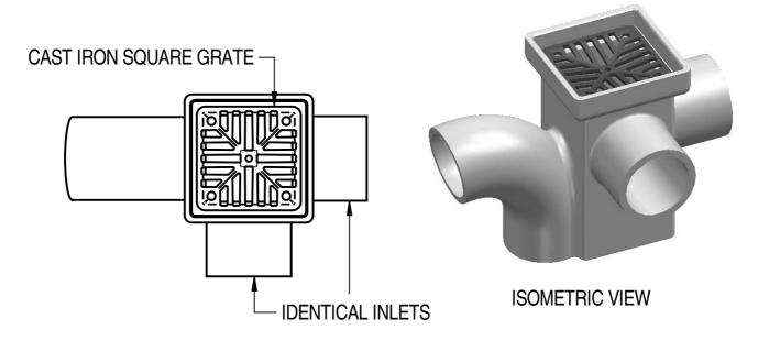
COMPLETE WITH CAST IRON SQUARE GRATE 150 x 150 (6" x 6") CODE KIG2C ALL DIMENSIONS IN mm
