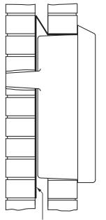
A polythene sheet 0.1mm thick or suitable cavity tray to be fitted by the builder
