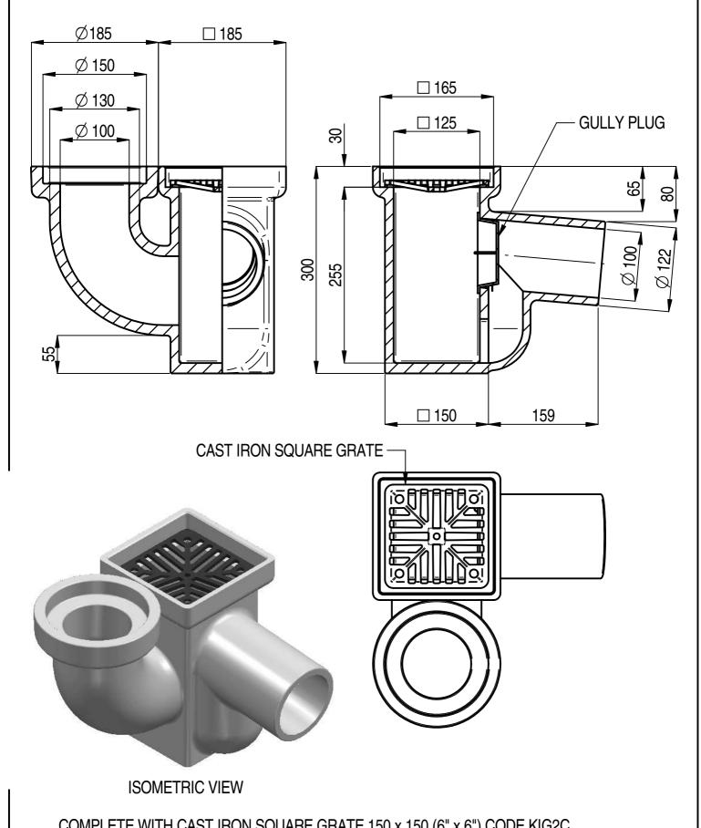
COMPLETE WITH CAST IRON SQUARE GRATE 150 x 150 (6" x 6") CODE KIG2C ALL DIMENSIONS IN mm
