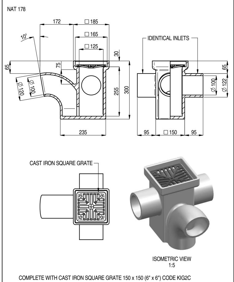
COMPLETE WITH CAST IRON SQUARE GRATE 150 x 150 (6" x 6") CODE KIG2C ALL DIMENSIONS IN mm
