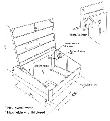
The installation pipe should enter the property as close as practicable to the outlet of the meter box, keeping to a minimum the pipework external to the dwelling. If necessary, the installation pipework (up to 22mm outside diameter) may be run behind the box in the space provided below hinge level
